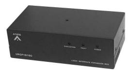
The URGP-16I16O is an extension unit for the IDA8-System, LAPG2T and ECS. The URGP16I16O provides those systems with 32 alarm inputs and outputs. Each input is monitored and can be programmed to trigger a digital audio message into a specific zone or group of zones. The URGP is linked to the System units through a RS232 /RS485 monitored serial link.
