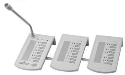
PPM-AS is an unidirectional addressable condenser paging microphone for IDA8 system. In accordance with BS5839, it is monitored by using the RS485 protocol over STP CAT5/6 cable with metal shielded connector, and transmits both audio and power from the paging console to the system units. The PPM-AS has 8 zone buttons with a sleek gooseneck microphone, providing durability and aesthetics in a slim, stable chassis.
