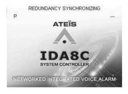
1. "P" or "S": if the device is the primary device, a letter P will be shown. If it is a secondary device, a letter S will be shown.
