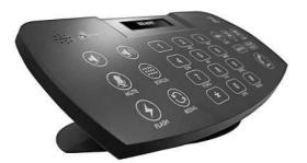
DIALER-DP dialpad is a touch dial, tabletop controller that connects to IDA8 or ECS processor. Users shall perform local and SIP call by connecting to either external telephone set with phone line or DIALER-DP with Ethernet connector.
