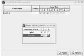
From the picture above, the logic output of channel 1~3 are selected. Click the [...] grid to open [Event Trigger] window.
