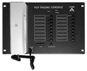
The PCP paging console is a wall-mounted heavy duty remote which is compatible with Ateis audio processor, The PCP console interconnects over a dedicated RS485 for power, audio and data transmit. The RS485 communication protocol with daisy-chain wiring can support up to 300m over CAT5 cable connection.
