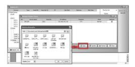
6. Select the desired URC-200 for updating by clicking [Selected] checkbox. Press [Update] to start updating procedure, which uploads the firmware program to the device's flash memory. There are progress bars for each URC-200 displaying the progress of the procedure. Once updating is finished, please press [Restart] to restart the device and make the change takes effect.
