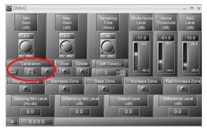
11. After the calibration is successful, the green LED will light up, and the DNM will start to work.
