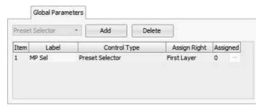
The URC-150AS settings of controlling the global parameters like changing master/sub presets. Users are allowed to create arbitrary number of items until reach the memory limitation which displayed on the bottom of window.
