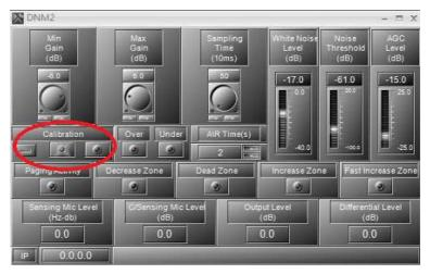
8. After the calibration is successful, the green LED will light up, and the DNM will start to work.
