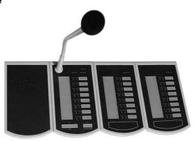
The PSC-AS microphone console is an unidirectional condenser addressable microphone which is compatible with all Ateis audio processor. Up to 32 x PSC-AS units can be connected using the daisy-chain wiring via RS485 protocol, and support up to 300M over a single CAT5 cable connection, the PSC-AS transmits both audio data and power supply to system units.
