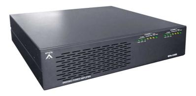
The BPA is a 2U 19" rack-mountable, 2-channel amplifier, transformer isolated for 100V, 50V, 8 ohm or 70V, 35V, 8 ohm loudspeakers. The 2 line inputs are with a balanced 3-pin XLR input and a balanced 3-pin phoenix input. The BPA amplifier range consists of five models: BPA-2060 (60W x 2),
