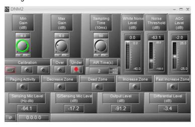
10.If the White Noise Level goes down to -40dB and the over LED is lighted up, this means the calibration has failed at this time, and the DNM received the sound too loud, please check:
