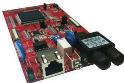
NET-C2, 1x RJ45 Port B &amp; 1x fiber Port A
