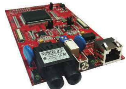
NET-C4, 1x fiber Port B &amp; 1x RJ45 Port A
