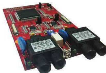
NET-C3, 2x fiber Port A &amp; Port B
