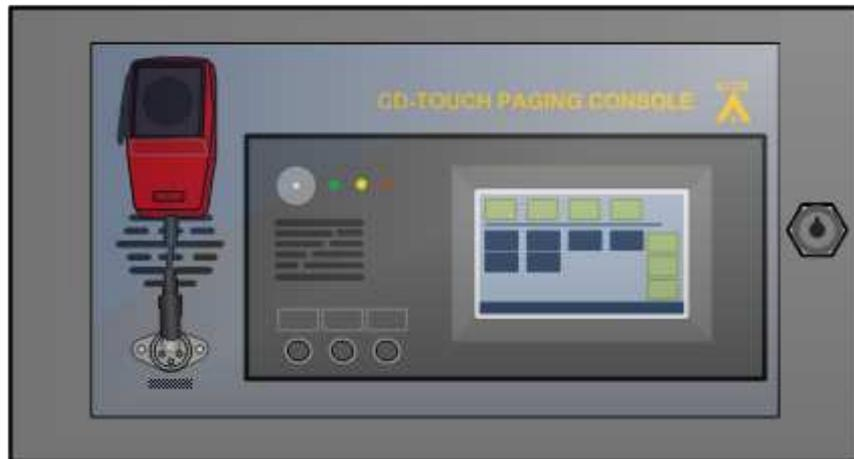
The PSSG2, CD-TOUCH paging microphone console is a man-machine interface which allows paging call, messages broadcasting and DSP matrix parameter control. DIVA8G2T can handle one PSSG2, CD-TOUCH unit connected to a secured bus. Its back-lit touch screen is designed for simple and user-friendly operating. Various operating levels with password protection make the PSSG2, CD-TOUCH a versatile device that fits well in a commercial shopping center as for an industrial high security environment.
