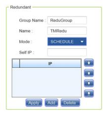
• Group Name: The group ID for the TerraManager using for redundancy purpose.
