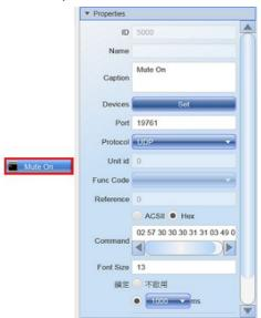
3. Click on the button to send the command. The example here is sending a "Mute" command.
