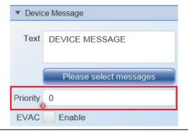
• EVAC: If the message is recorded for emergency use, tick the Evac checkbox. The Evac indicator
